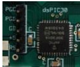
The top 2 pins are PGD and PGC (which you need to short together In order to perform the reset action)
